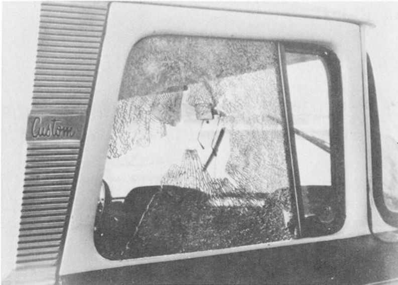
FIG. 1—Tempered plate glass window of door on passenger side of pickup truck with defect caused by bullet fired from large caliber handgun.
